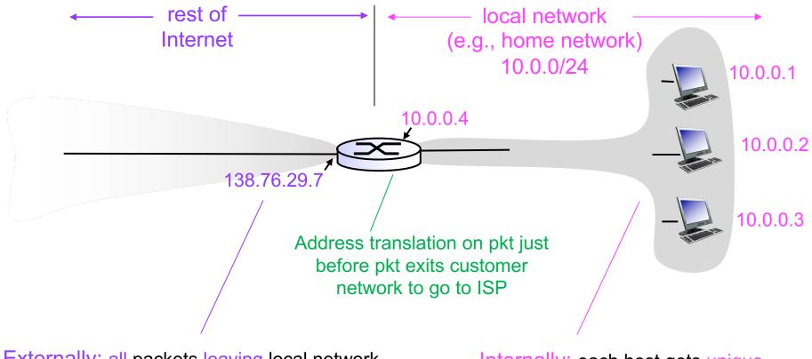
Externally: all packets leaving local network have same single source NAT IP address: 138.76.29.7, different source port #s
