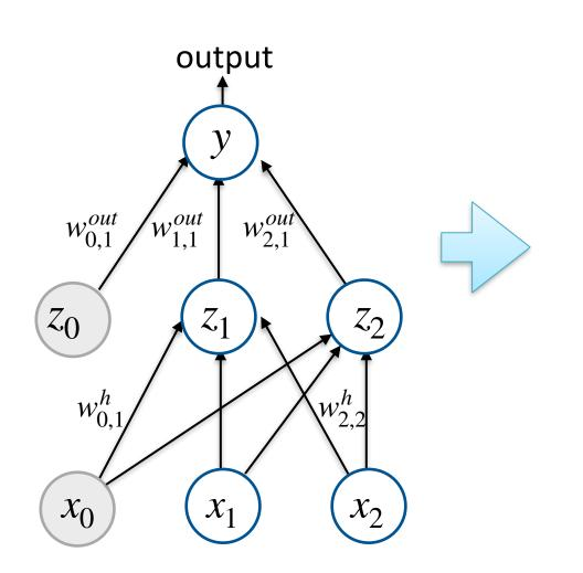
Each element of  $\mathbf{z}$  is  $z_i$  and is generated by the sigmoid activation to each element of  $\mathbf{W}^h\mathbf{x}$
