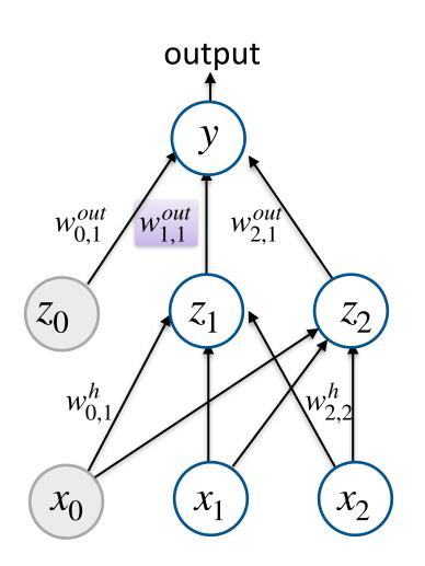
$$\frac{\partial L}{\partial w_{1,1}^o} = \frac{\partial L}{\partial y} \cdot \frac{\partial y}{\partial w_{1,1}^o}$$
