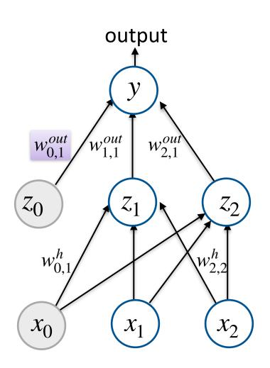
$$\frac{\partial L}{\partial w_{0,1}^o} = \frac{\partial L}{\partial y} \cdot \frac{\partial y}{\partial w_{0,1}^o}$$
