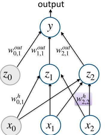
$$\frac{\partial L}{\partial w_{2,2}^h} = \frac{\partial L}{\partial y} \cdot w_{2,1}^o \frac{\partial z_2}{\partial s} \frac{\partial s}{\partial w_{2,2}^h}$$
