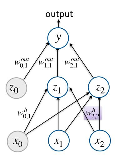
$$\frac{\partial L}{\partial w_{2,2}^h} = \frac{\partial L}{\partial y} \cdot \frac{\partial y}{\partial w_{2,2}^h}$$
