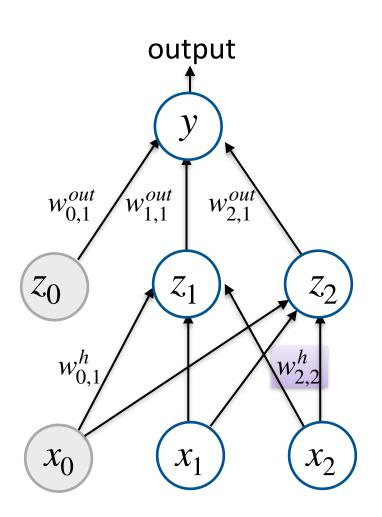
$$\frac{\partial L}{\partial w_{2,2}^h} = \frac{\partial L}{\partial y} \cdot w_{2,1}^o \frac{\partial z_2}{\partial s} \frac{\partial s}{\partial w_{2,2}^h}$$
