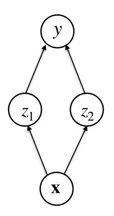
$$\frac{\partial y}{\partial \mathbf{x}} = \frac{\partial y}{\partial z_1} \cdot \frac{\partial z_1}{\partial \mathbf{x}} + \frac{\partial y}{\partial z_2} \cdot \frac{\partial z_2}{\partial \mathbf{x}}$$
