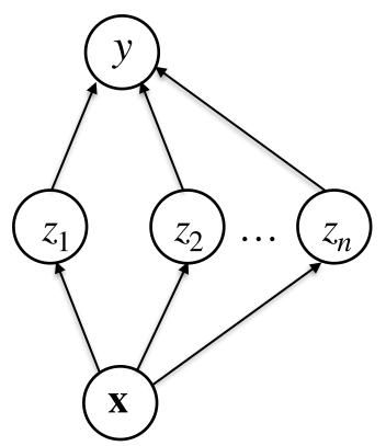
$$\frac{\partial y}{\partial \mathbf{x}} = \sum_{i=1}^{n} \frac{\partial y}{\partial z_i} \cdot \frac{\partial z_i}{\partial \mathbf{x}}$$
