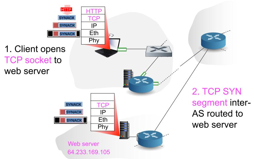
3. Web server responds with TCP SYNACK and client replies with TCP ACK. Connection established!
