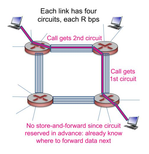
Q: what is end-end transmission delay? L/R seconds
