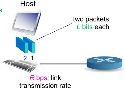
$$\frac{\text{Transmission}}{\text{delay}} = \frac{\text{Time to transmit } L\text{-bit}}{\text{packet into link}} = \frac{L \text{ (bits)}}{R \text{ (bits/sec)}}$$
