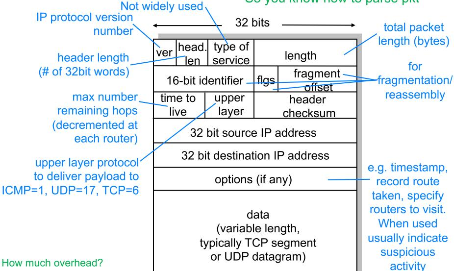
20 bytes of TCP 20 bytes of IP
