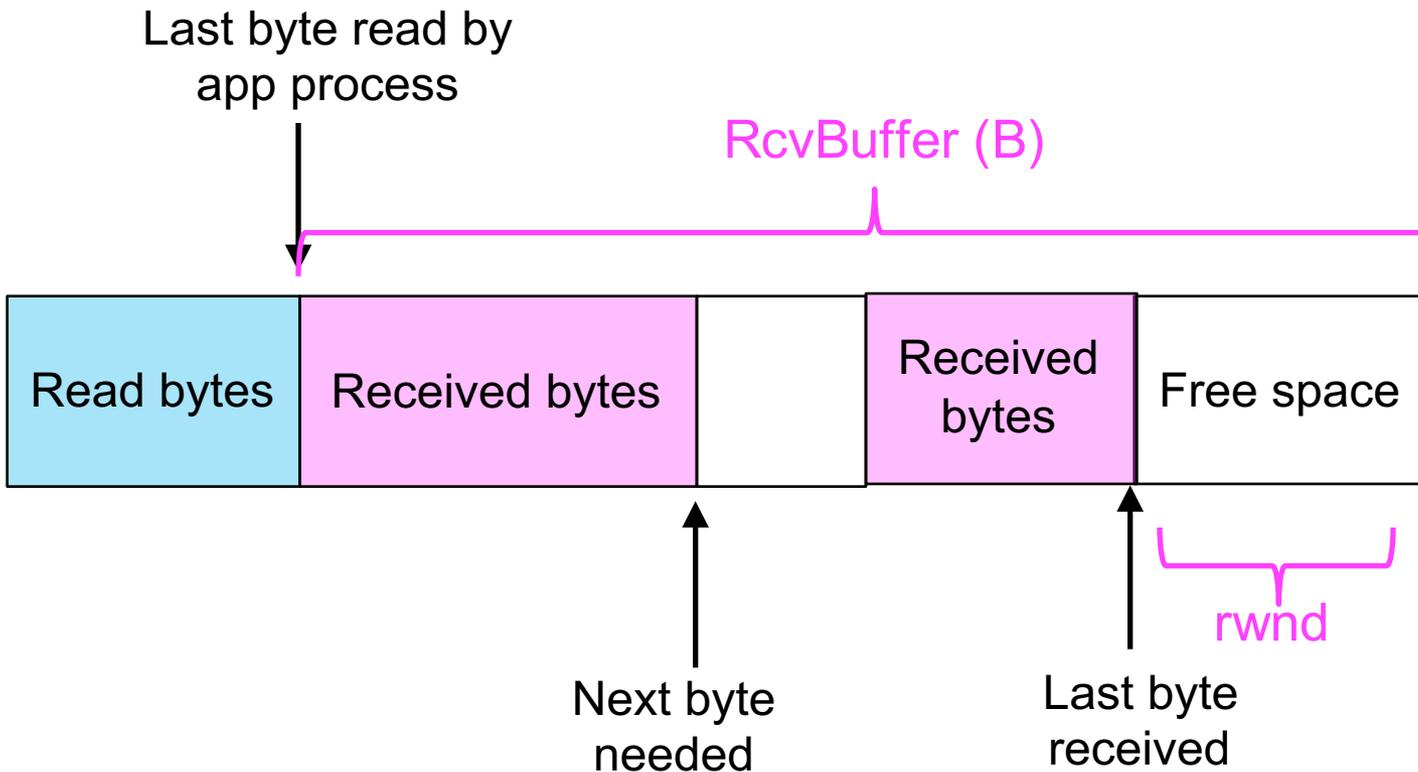
$$rwnd = B - (\text{last byte received} - \text{last byte read})$$
